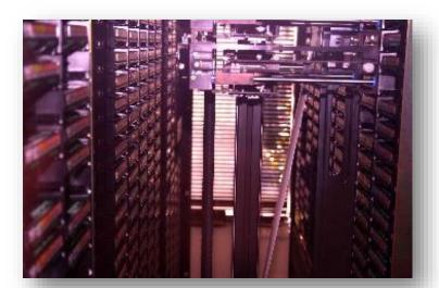
Discovery Reply MAM, allows the near-line archival and off-line management of digital data onto LTO5 tapes.
